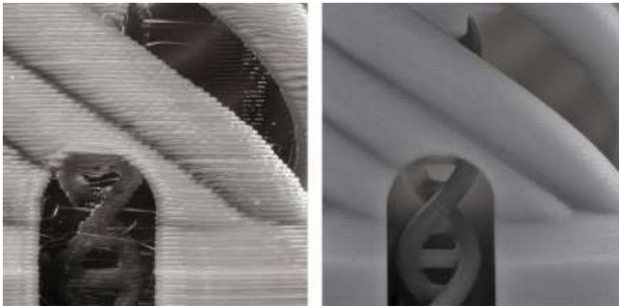
Figure 7 – Comparison of manufacturing the same object using different processes: FFF (left) and DLP (right).
