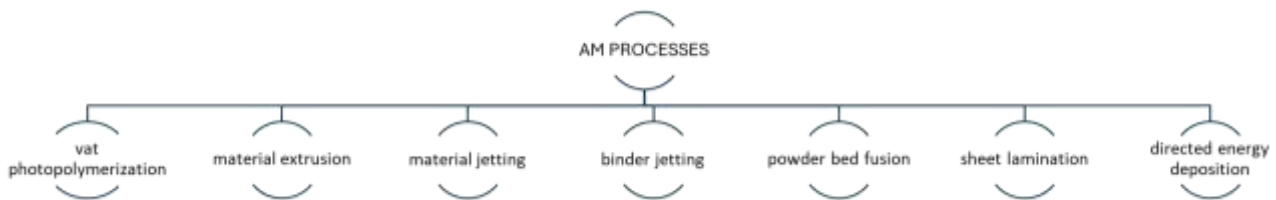
Figure 3 – Classification of AM processes according to the layer addition principle.
