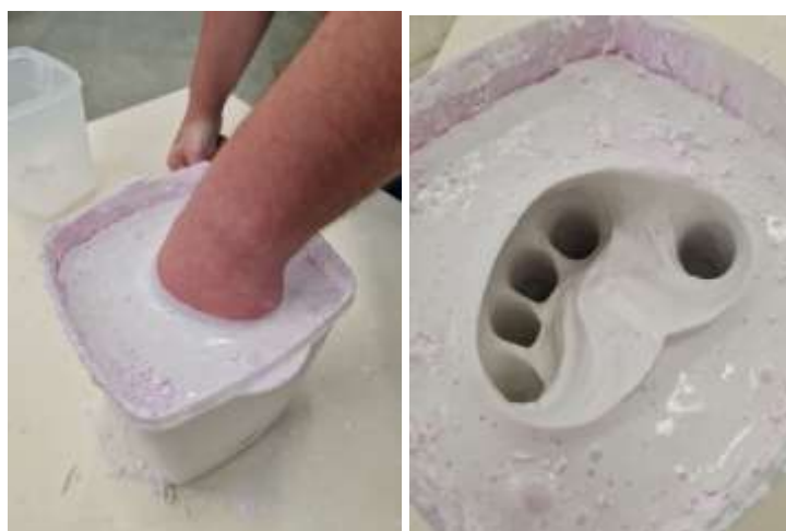
Figure 13 – Obtaining alginate molds: a) waiting for setting time; b) result after removing the hand.
